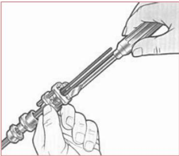
Fully slacken the two screws, slide the crimping plate over the conductors and up to the seal pot. The slotted base plate swivels around the cable under the seal pot then tighten the two screws evenly. This will drive the stub cap or disc fully into the seal pot recess and secure it into position by indenting the brass seal pot wall in three positions. Slacken and remove tooling
