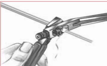
Alternatively if no ringing tool is available the length can be stripped as above and pliers used to stop the stripping action and create a straight neat end.
