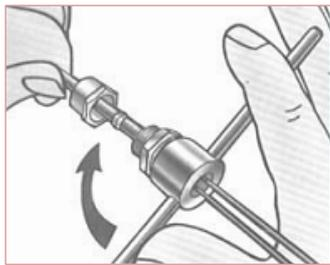
Leave the gland nut and compression ring on the stripped end of cable and position the seal pot in the recess within the gland body and screw the gland into the Pot wrench. Finger tightness is sufficient at this stage. As you apply downward pressure the pot will create a thread on the cable sheath
